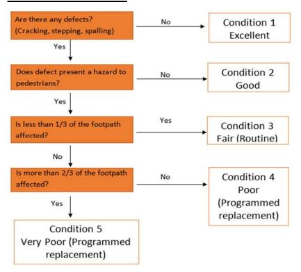
This flow chart has been used to determine the condition of each section of footpaths within Warren Shire Council.
